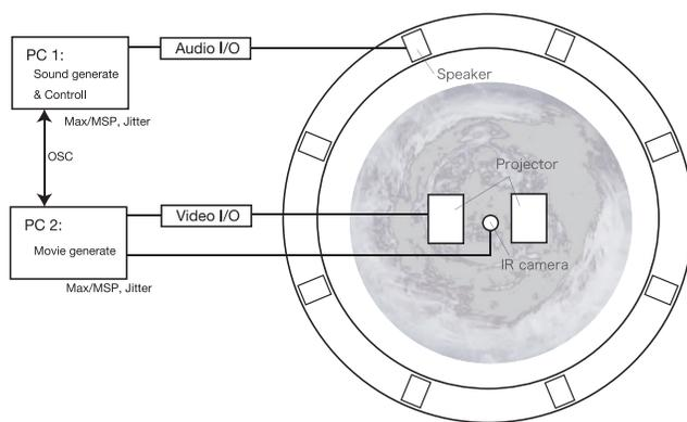
Figure 2. System diagram.
